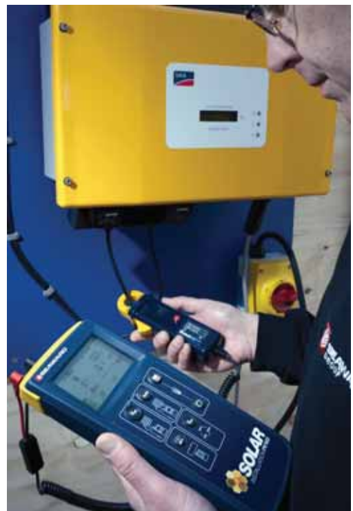
Diagnostic solution: Seaward's multi-function PV 100 electrical tester is one of the products on show at Ecobuild
