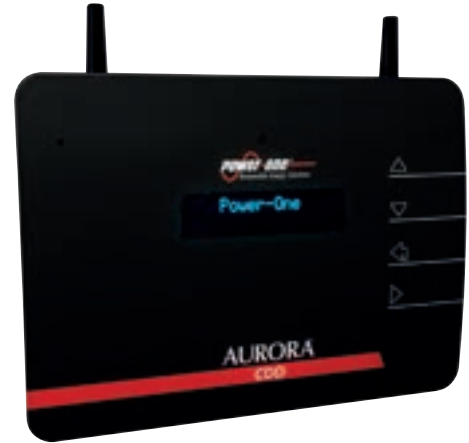
Quick thinking: Power-One says its Aurora CDD monitoring device enables installers to identify PV problems in rapid time
