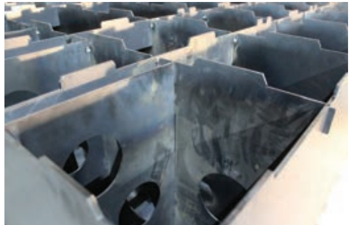
Space saving: Fair Energy's buffer tank design offers multiple benefits due to its unique rectangular shape, says R&D engineer Ben White
