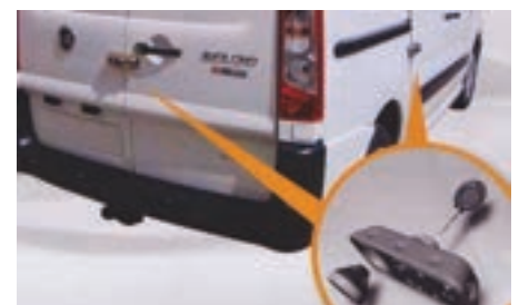
Doubling up: Installers should always back up the standard locks supplied on vans, advises Trade Skills 4 U
