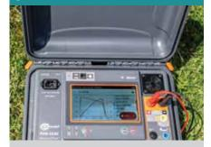
THE Sonel PVM-1530 and associated equipment comply with IEC 61557 and IEC 61010 safety standards and have the relevant CE declaration. IEC 61010-30 qualifies PV panels as belonging to the CAT III measurement category and, crucially, with its high CAT III 1500V DC measurement category, the meter can measure panels working at voltages up to 1500V.
